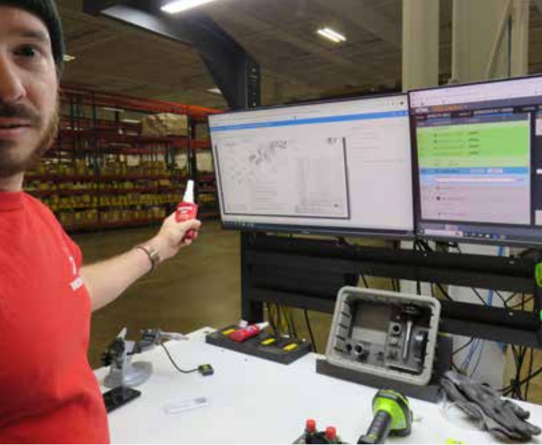
Top Left: The automated manufacturing process Jack Matthews is developing has sensed he has picked up Loctite 263, not the other Loctite on the table, hence the green status of that step. Right: Each step of an assembly process provides specific instructions and senses when the correct tools are picked up. Below: Automated part measurement validation system, accurate to .0000001 inch.
