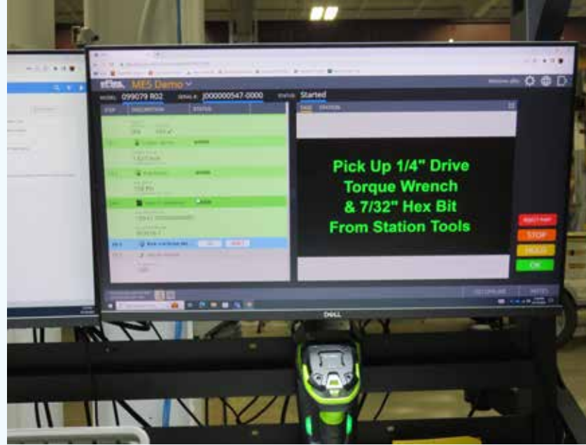
Top Left: The automated manufacturing process Jack Matthews is developing has sensed he has picked up Loctite 263, not the other Loctite on the table, hence the green status of that step. Right: Each step of an assembly process provides specific instructions and senses when the correct tools are picked up. Below: Automated part measurement validation system, accurate to .0000001 inch.
