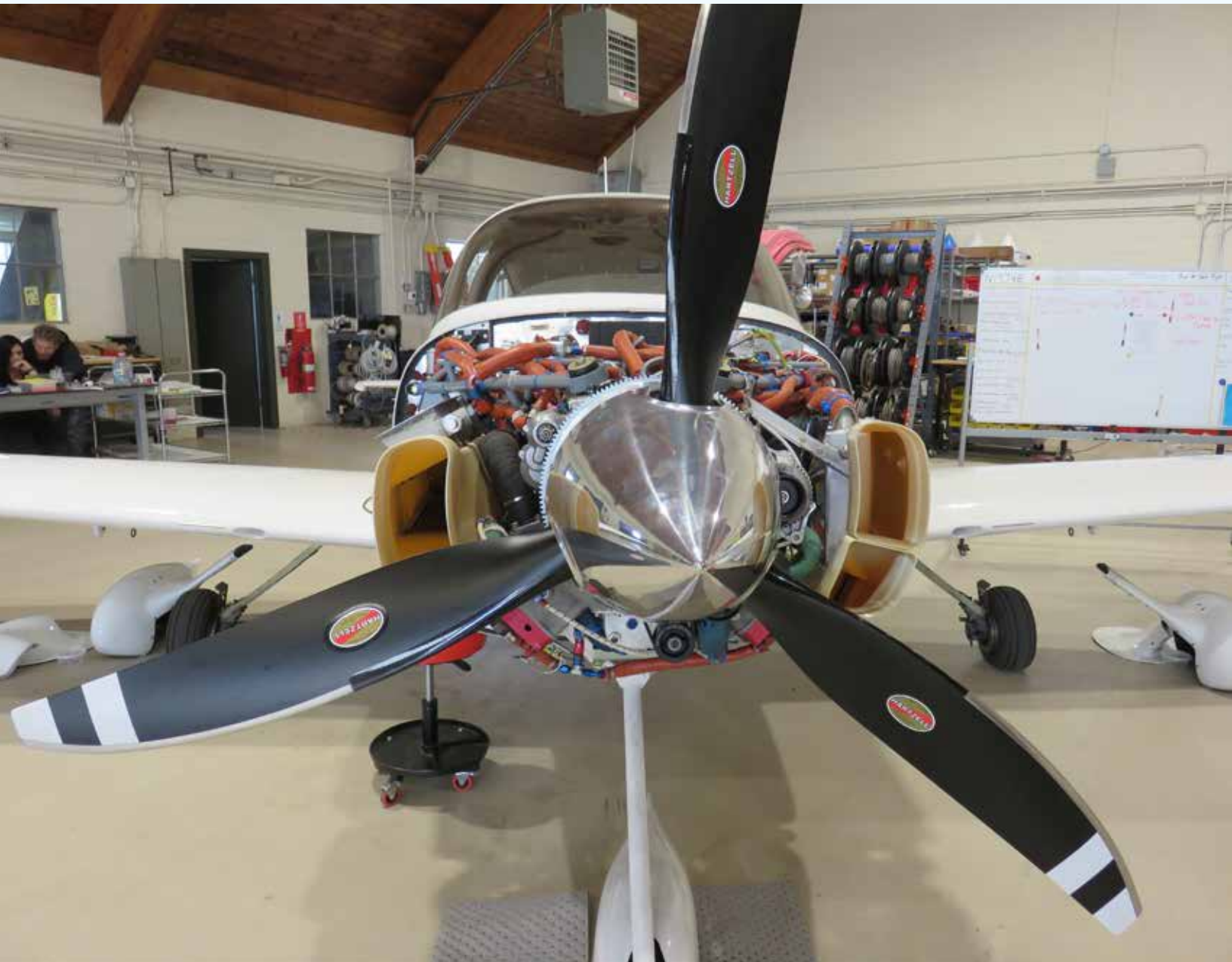
The DHK180 as installed "upside down" in a Cirrus SR20 for flight testing. The engine will run in any orientation and can be used in a pusher configuration without modification.
