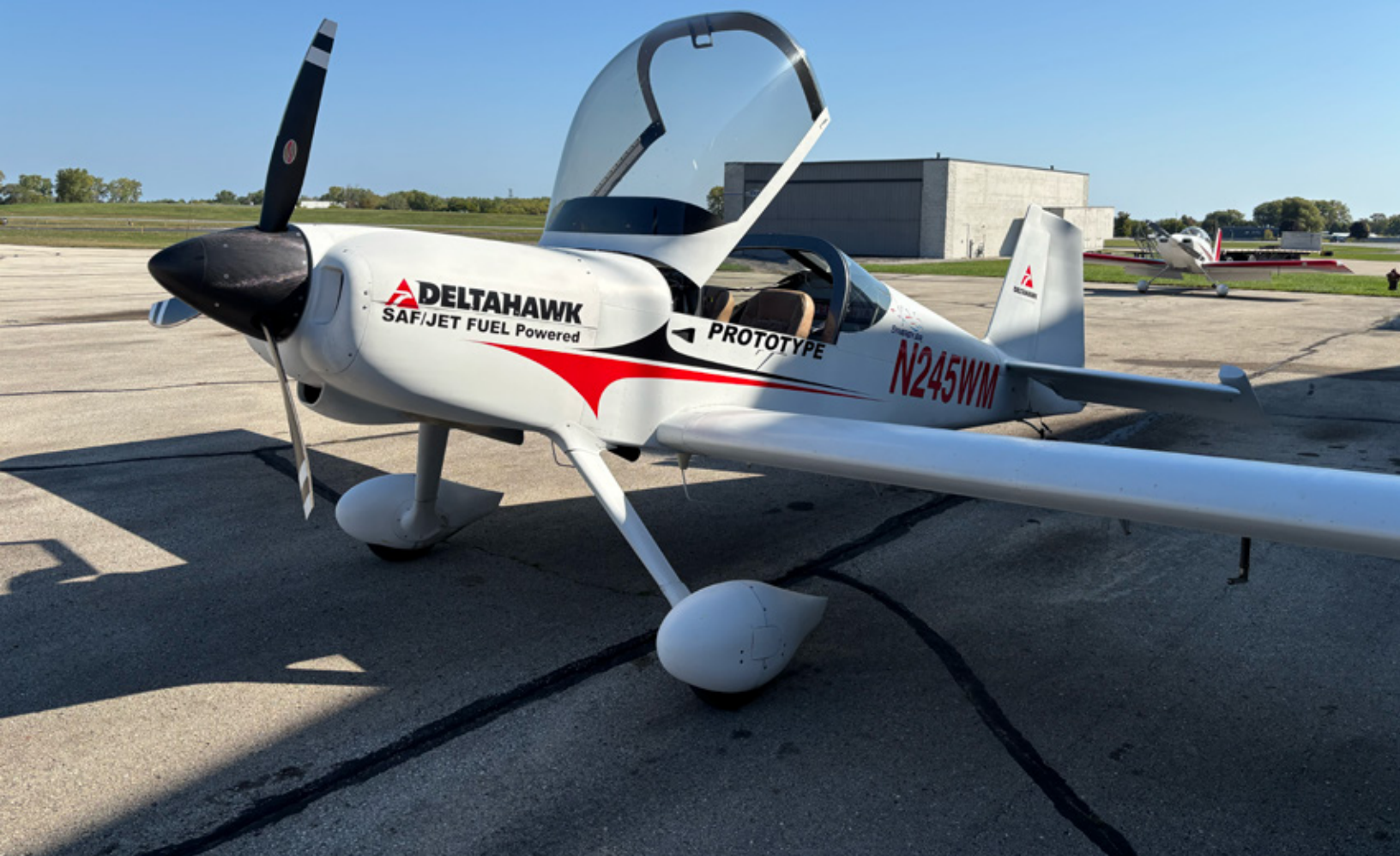
Craig Saxton's Van's RV-14 with the DHK180 engine and MT prop at the DeltaHawk headquarters for testing and documentation.
