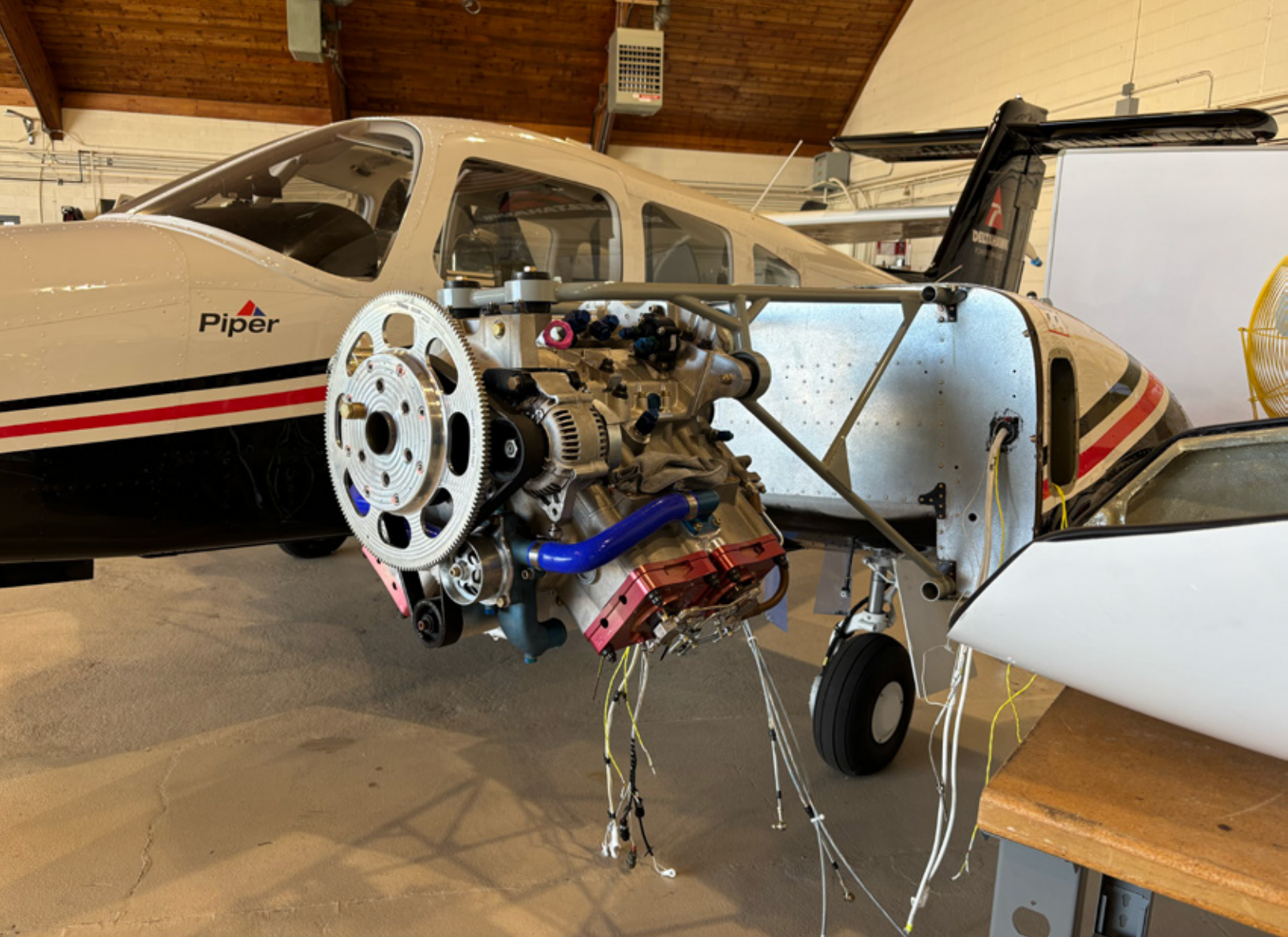
The beginning of an installation of the DHK180A4 on the PA-44 Seminole DX.
