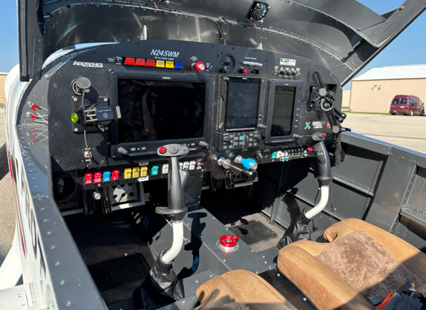
The panel of Craig's RV-14. Note the absence of a mixture control. The switch on the left goes down to heat up the glow plugs for start, then up for start.
