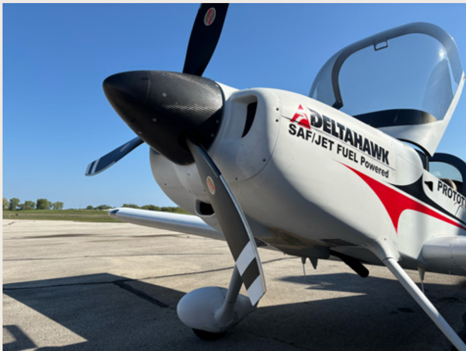
DeltaHawk cowlings will have two primary air intakes with dividers that direct air to the engine and three heat exchangers, engineered to minimize resistance to send the right amount of air to each component.
