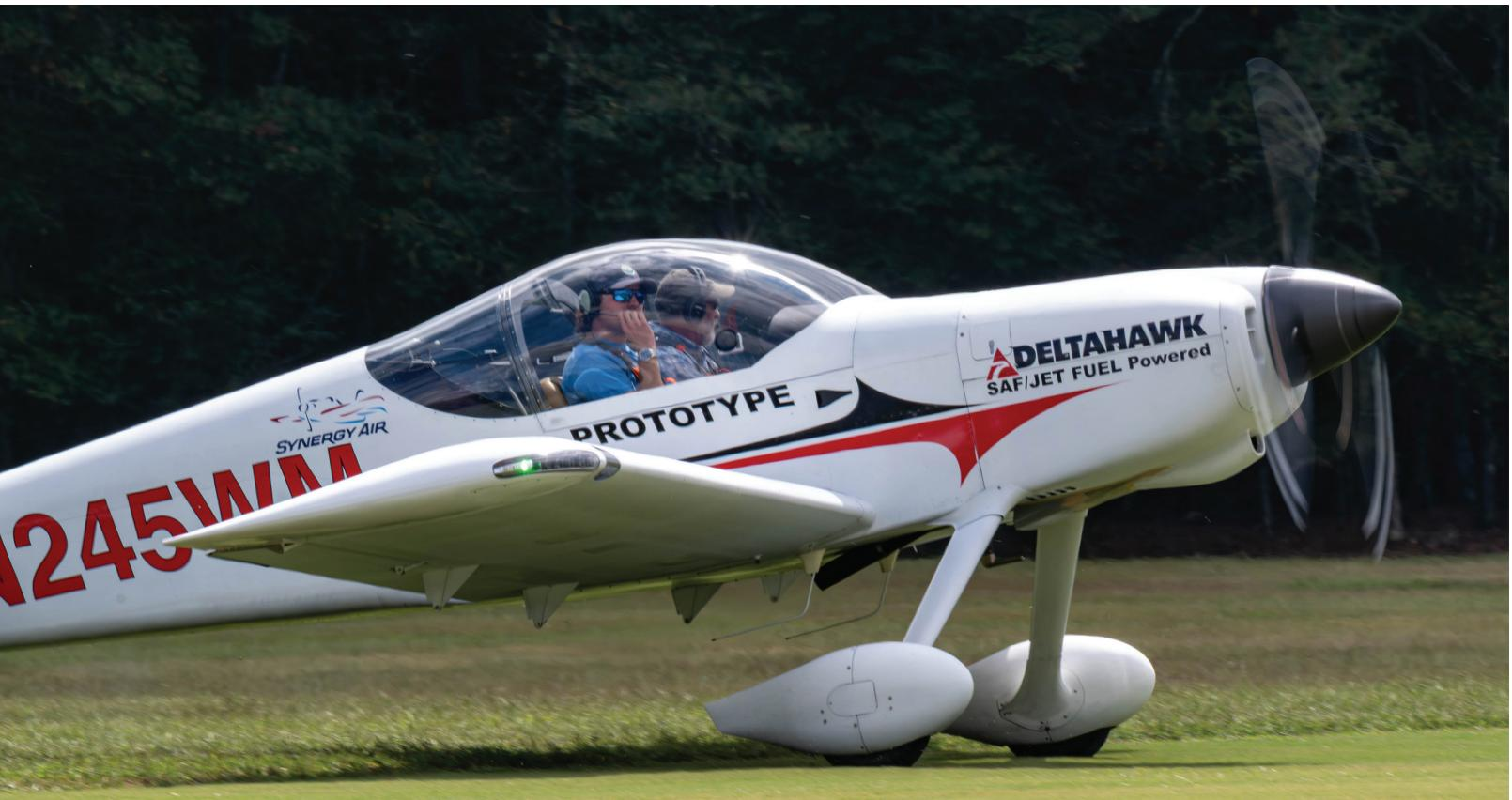
DeltaHawk engines excel economically, delivering 35 to 40 percent better fuel efficiency than comparable avgas engines — savings you'll see right away at the pump. When flying on a max range profile (167 knots true airspeed), the DeltaHawk burns 7 gph. With no wind, this aircraft flies for about 27.4 statute miles (23.9 nm) per gallon. To top it off (pun intended), Jet A fuel averages about \$1 cheaper than 100LL at most airports Craig frequents.
